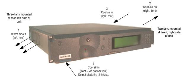
Figure 2.2: Air Path Through the Enclosure
